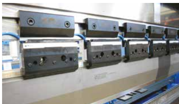
European style pneumatic clamping with intermediates (H=100mm) with vertical tools insertion.
