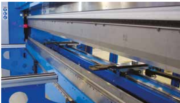
Wila Style manual clamping (standard or hardened).
