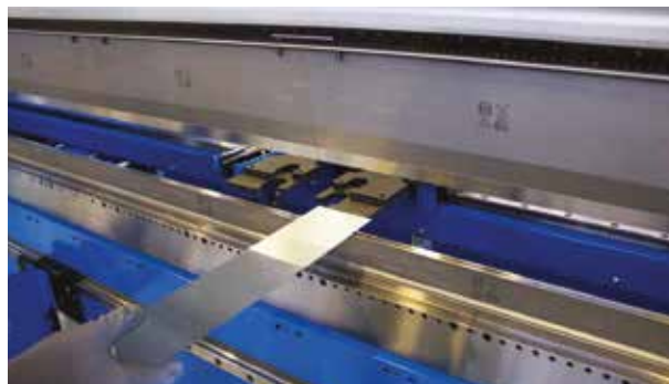
Wila style Hydraulic clamping (standard or hardened – here with STL option).
